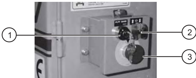
Figure 2-4A. Base Control Box and Labels (Located at rear of hydraulic/electric side cabinet)
