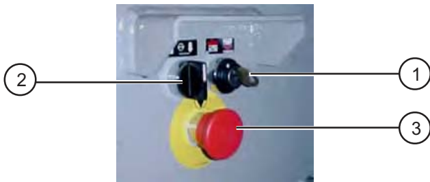
Figure 2-4A. Base Control Box and Labels (Located at rear of hydraulic/electric side cabinet)
