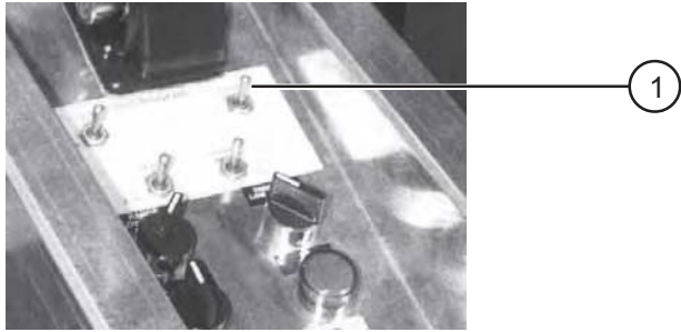
Figure 2-8A. Outrigger Controls On Operator's Control Box
